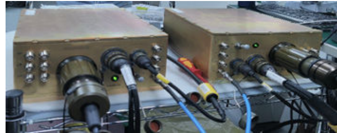
Figure 5 6 channels RFoF militarized phase-matched system
