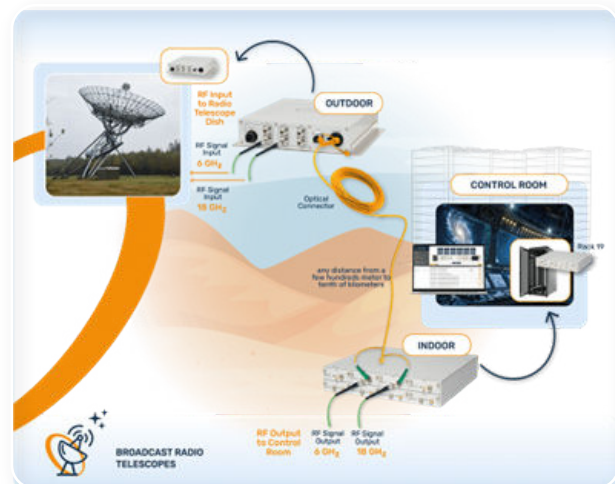
Figure 10 Overview of RF over Fiber for Radio Telescope
